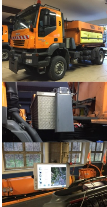
Pictures: Gritting vehicle of AM Greding (top), sensor mounted on the gritting vehicle (centre) and monitoring on a tablet in the driver's cab (bottom) – Source: BAST
