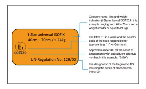
Appropriate marking must be affixed on child restraint systems with vehicle-specific approval in accordance with UNECE Regulation 129.
