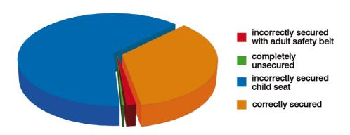
A step towards the reduction of misuse is the introduction of the IsoFix anchorages. IsoFix is a rigid connection of the child restraint system and the car via two standardized attachment points. This system facilitates the installation of child seats into the car and reduces potential misuse. In addition, the IsoFix protective system has a further anchoring point in the vehicle to prevent the child seat from rotating. Here, a support leg or a top tether can be used.
