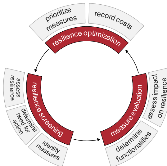
Fig. 3 Resilience management concept. The elements relevant for the proposed methodology are highlighted in red based on Deublein et al. (2018)
