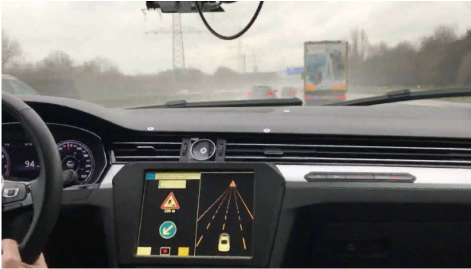
Fig. 6 RWW Service displayed on the prototype HMI [12]
