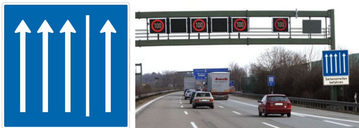
Fig. 4 a) sign 223.1 “use hard shoulder”; b) example of temporary use of hard shoulder (Picture: Autobahndirektion Südbayern, edited by BAST)
