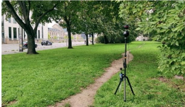
Fig. 1. Setup for measuring audio-visual road traffic scenes with Ambisonics microphone (Zylia ZM1), sound level meter (NTI XL2) and 360° camera (Insta360 Pro II)
