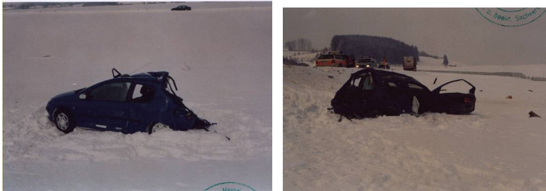
Figure 16: Case 11 - Final position of vehicle, driver's (left) and passenger's side (right)
