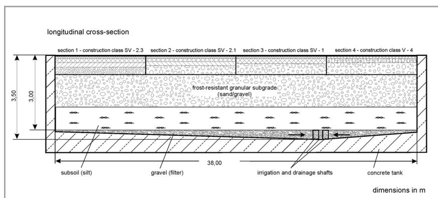
Cross-section of the asphalt pavement test track with four different pavement constructions according to the German guideline RStO
