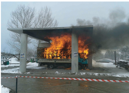
Scenario-oriented research: Fire under a bridge
