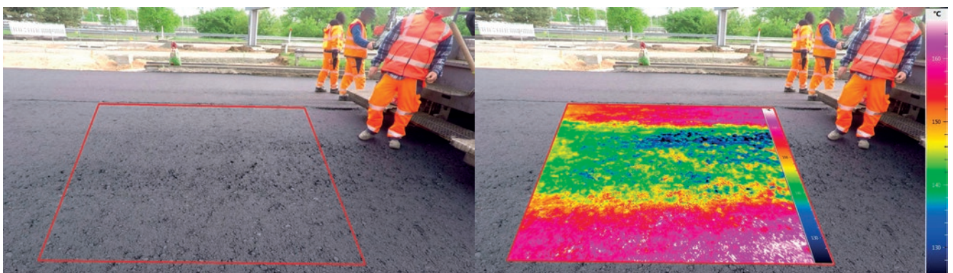
Tested image detail in the visual range (left) and the infrared range (right)
