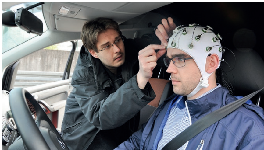
EEG monitoring in BAST's research vehicle
