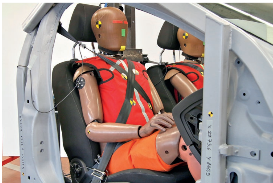
THOR sled test with four-point belt system
