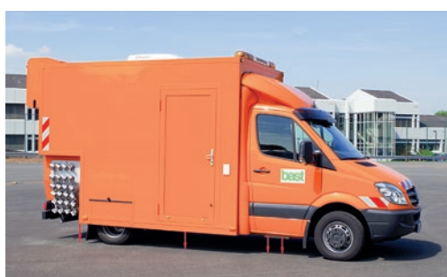
Methods to detect longitudinal unevenness: MEFA (multi-functional detection system for road surface analysis) (left) and planograph (right)
